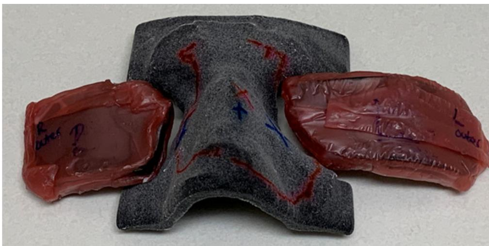
*This image shows the TPU01 bolus with custom lead blocks wrapped in wax. The purpose of the wax was to reduce electron side scatter.*
