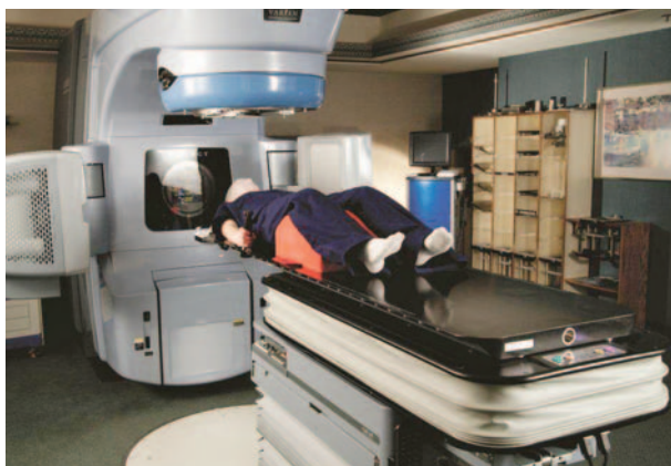
The Protura Robotic Patient Positioning System fully enables IGRT by providing sub-millimeter corrections with 6 degrees of freedom.
