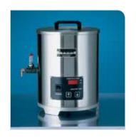
This highly-durable production melter has a heavy-gauge stainless steel inner and outer wall construction with full-wrap ceramic heaters. The heated ball valve dispenser helps prevent nozzle blockage. The digital readout provides a constant temperature reference, along with programmable tank and dispenser temperature settings. It can be used with either low-melt or medium-melt alloy.
