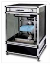
The Compu-cutter uses precise, digitized radiograph outlines to cut shielding block molds with  $\pm 1$ mm accuracy. Block outlines can be manually digitized or transferred from treatment planning systems. A window based program digitizes and stores files for future reference or quick modifications. The Compu-cutter can 'flip' images for fast AP/PA or L/R lateral blocks, or easily change any parameter without re-digitizing. A four-axis, CNC cutter is safely enclosed in our self-contained model.
